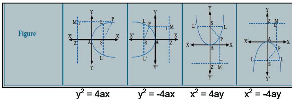
**Note:** In the figure above, A represents the vertex, S represents the Focus, LL' represents the Latus Rectum and Line MZ represents the Directrix to the parabola.
